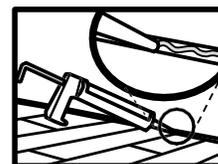
After installing planks and before installing trim, remove all spacers. Create a water tight spacing applying 3/8" PE foam backer rod and 100% flexible silicone sealant along the entire perimeter of room and around fixed objects and transitional moldings. Do not use acrylic sealant.
